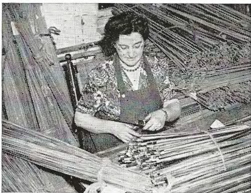
Montague for years has imported special growth Tonkin cane from far-off China for Montague bamboo rods. Here the cane has been split and is being tied into matched sections.
